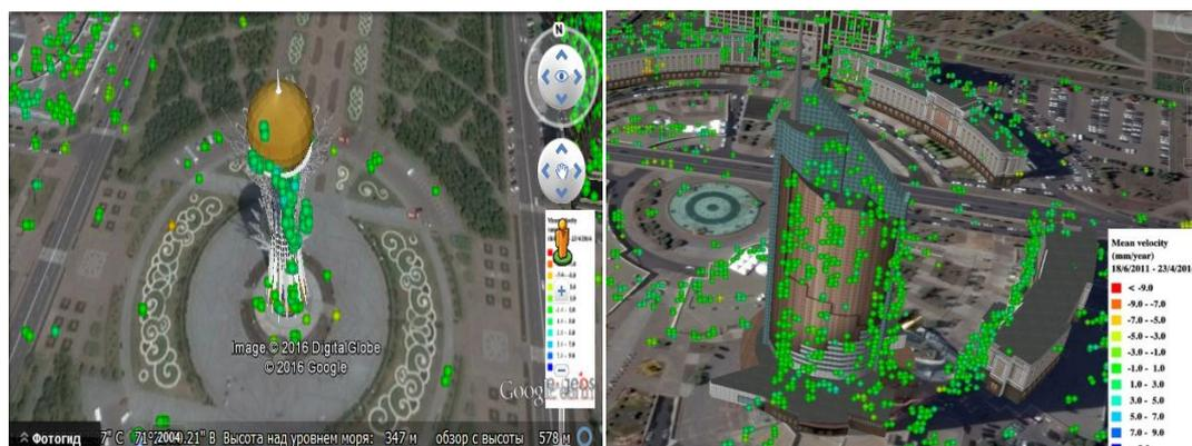
Figure 1 - Sustainable reflectors of radar signal detected on buildings "Baiterek" and "Transport Tower" of Nur-Sultan city with background from Google Earth
